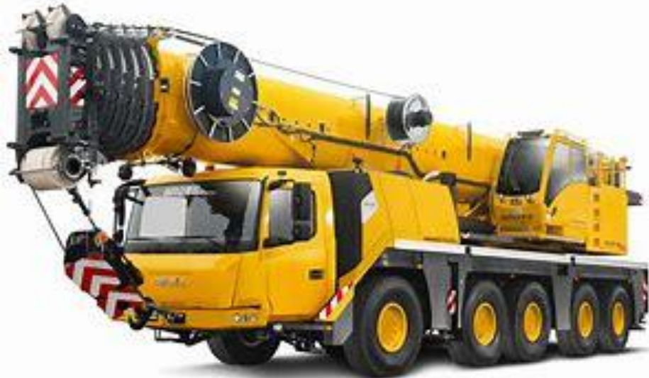
GROVE GMK 5150 30' W on outriggers 14' Counterweight swing 9'6" W x 41'3" L x 13'1" H 106,867 pounds + 98,000 lbs. counterweight
